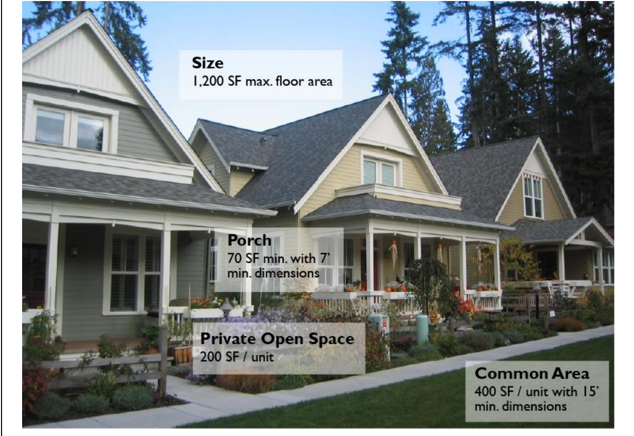
Figure 17.21.030(A)(1) Cottage housing example with key standards.
