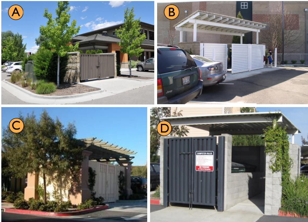
Figure 17.22.260(C) Acceptable trash screening enclosures.
